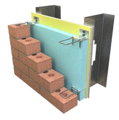
\*\*\*Anchor can be installed Horizontal or Vertical.\*\*\*
